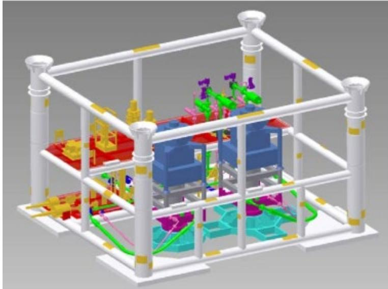
**Figure 3 - Wellhead Protection Structure (WPS)**
