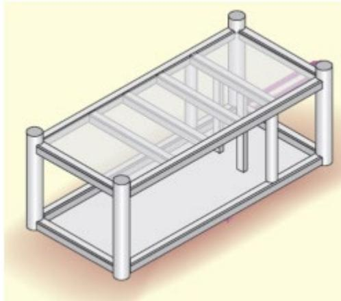
**Figure 5 - Subsea Umbilical Distribution Skid (SUDS)**
