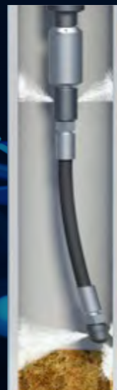
Pipetech scale remediation tool
