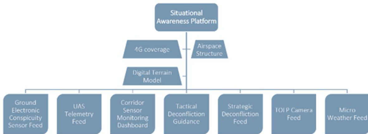
Figure 14: Components of a situational awareness platform to enable BVLOS operations within a TMZ
