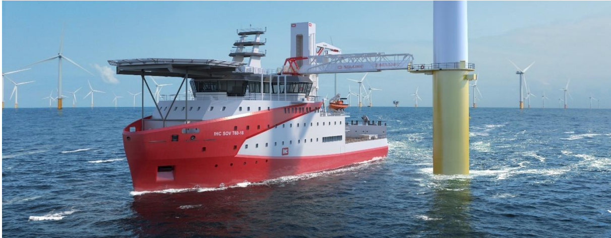
Figure 3-2 SOV with walk-to-work system at a turbine (source: Royal IHC )
