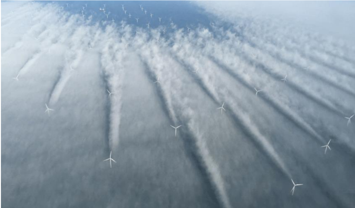
Figure 5-2 Aerial picture of the Horns Rev II wind farm, in which the wind turbine wakes are visualised by low hanging fog that is mixed into the wake region (source: Bel Air Aviation Denmark-Helicopter Services )
