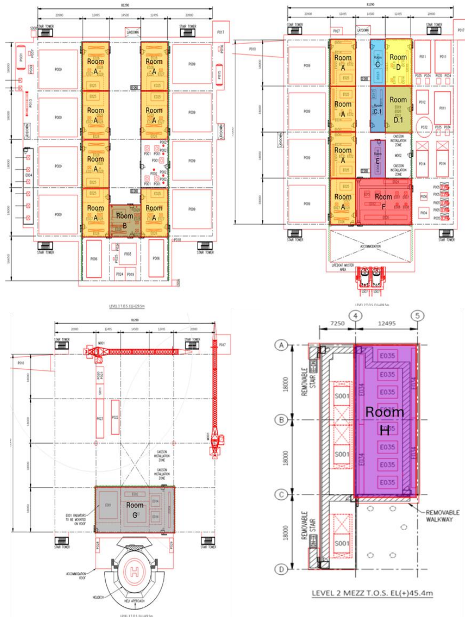
Figure 9 Rooms categorisation for HVAC requirements
